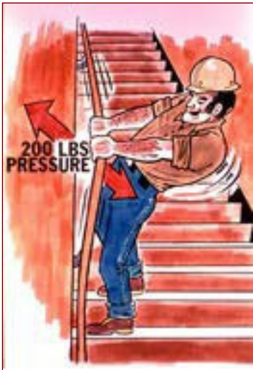
Figure 8-10 Guardrail Lateral Force
